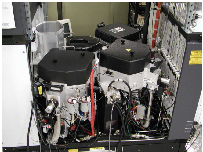
Figure 2 CVD-tool P5000 with chambers for post-treatment of dielectric and cap deposition
