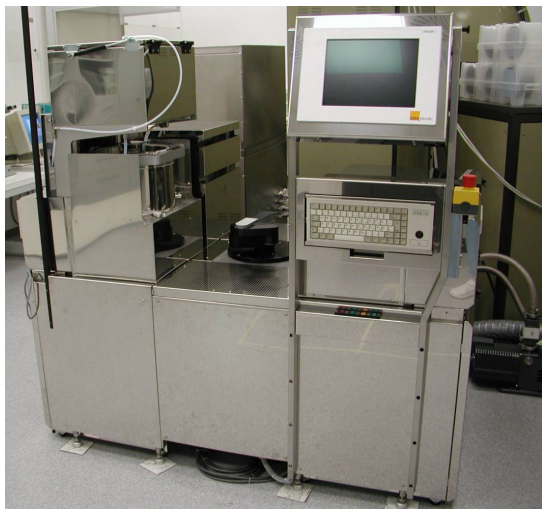
Figure 1 Spin on tool for deposition of dielectrics provided by SÜSS MicroTec
