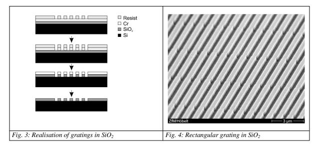
The rectangular gratings are fabricated using e-beam lithography and dry etching (Fig. 3). The grating pattern is transferred from the photoresist into a chromium layer (thickness 20 nm). This layer is used as a hard mask to dry etch a SiO<sub>2</sub>-layer on top of the actuator wafer, which defines the height of the grating. Figure 4 shows a SEM-Picture of such a grating.
