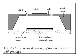
a PECVD process in order to fabricate a barrier between the glass and the driving electrodes. The 1  $\mu$ m thick metal layer for electrodes and wiring is sputter deposited and patterned.
