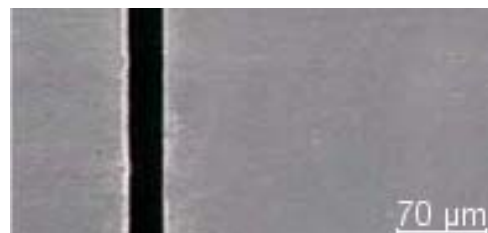
Fig. 4 Virtually absent heat-affected zones adjacent to fs-laser cut trench.
