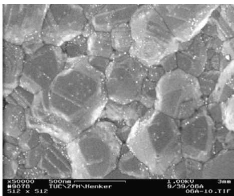
Fig. 3 Grain morphology of pure Cu film, SEM image
