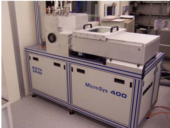
Fig. 2: MicroSys400 with the load lock on the right side
