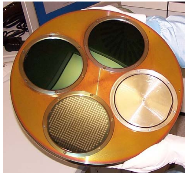
Fig 4: Carrier for 5-inch wafers. On the right the indentation with He channel in the middle and a viton gasket, on the left a diode wafer after plasma etching.
