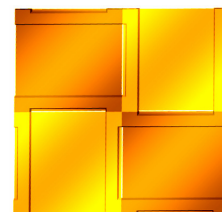
Fig 3: 90°-twisted aligned chips to prevent a preferred deflection of the wafer.
