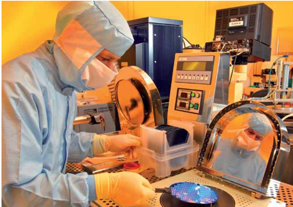
Fig.1: View into the new clean room facilities, equipment for depositing photo resist
