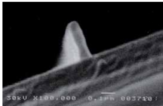
Fig.1: SEM-picture of a gate electrode of a sub-50nm-MOS-transistor
