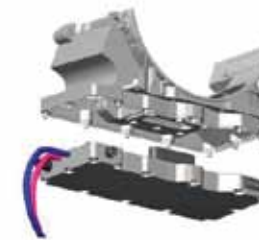
Fig.5: Partial integration of the power electronic system in the automobile gear unit (EfA-project). Figure from ZF Friedrichshafen AG
