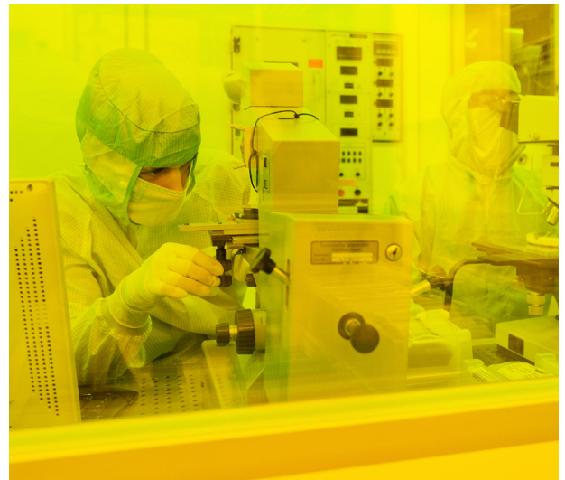
Fig. 1: Wafer inspection within the lithography clean room
