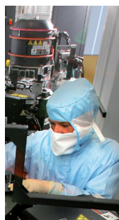
Fig. 2: P5000 used for deposition of Copper
