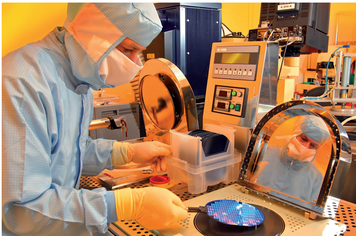
Fig. 1: View into the new clean room facilities, equipment for depositing foto resist
