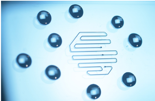
Fig. 2: Laser-micromachined microfluidic channel structure as part of a lab-on-chip system
