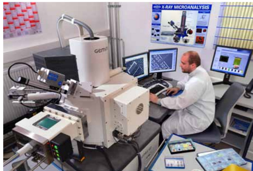
Sven Haas of the Center for Microtechnologies is examining under the scanning electron microscope micro-mechanical silicon structures of minute dimensions less than a micrometer. Photo: Wolfgang Thieme
