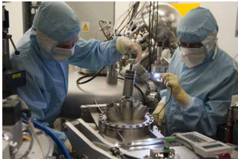
Dr. Thomas Wächtler and Dr. Jens Erben at the ALD cluster unit with integrated XPS analysis system for the in-situ characterization of nanometer-thin layers. Photo: Ralph Kunz
