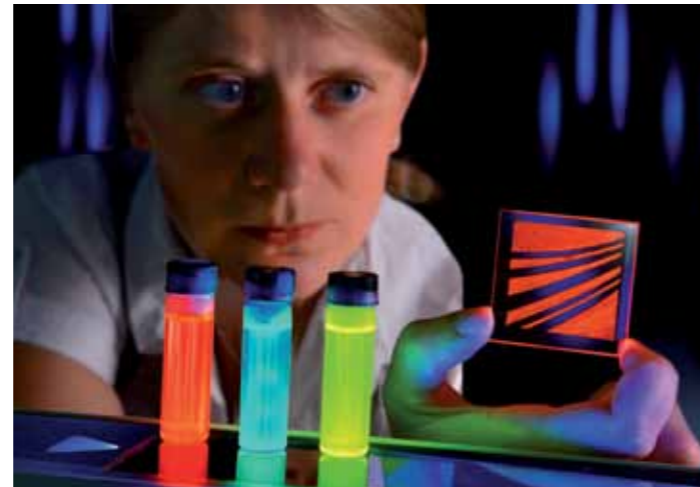
Chemical Engineer Dr. Kathleen Heinrich shows a sample body which is layered with quantum dots, i.e. nanoscopic semiconductor particles. When the tiny semiconductor particles are excited with UV light, they begin to fluoresce. What color the emitted light has depends on the size of the particles. If in some places a stress acts on the material, this fluorescence stops. Therefore, the affected areas remain dark when excited by UV light and point to the mechanical load. Photo: Wolfgang Thieme
