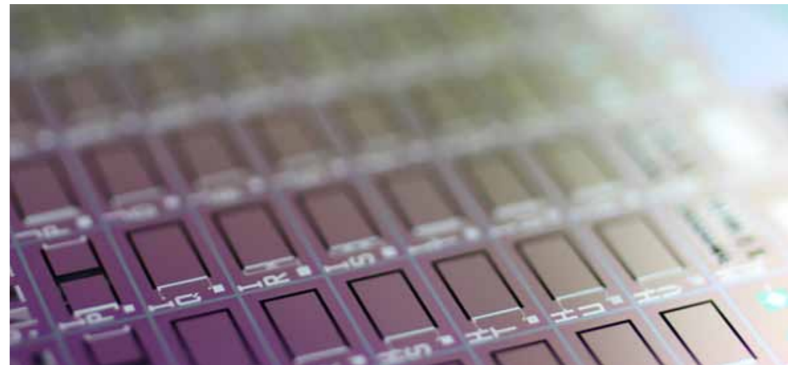
Fig. 1: PiezoMEMS at wafer level. PDIGs with integrated piezoelectric aluminum nitride.
