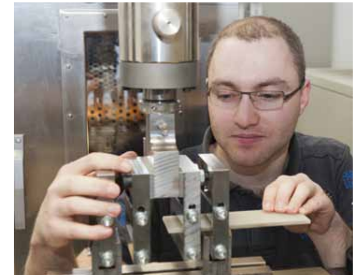
John Brückner of the workgroup led by Prof. Wunderle testing fiber-reinforced plastics in the 4-point bending test. Photo: Ralph Kunz
