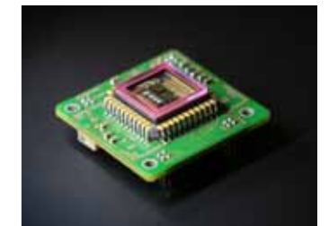
Fig. 9: Gyro prototype (ASIC on top of MEMS chip).
