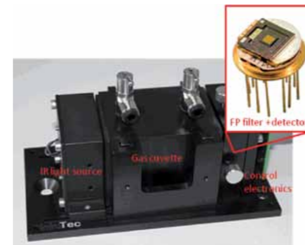
Fig. 3: Microspectrometer demonstrator setup based on MEMS FPI by courtesy of InfraTec GmbH Dresden
