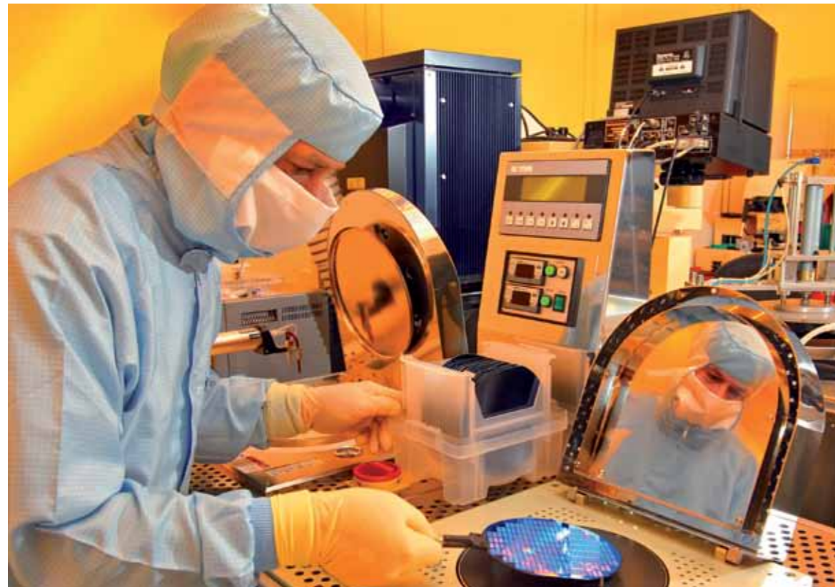
Fig. 1: View into the new clean room facilities, equipment for depositing foto resist
