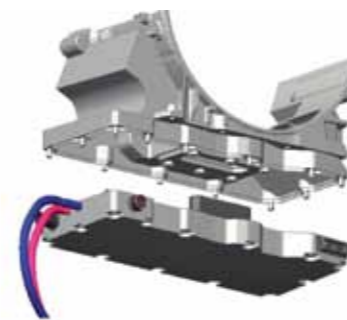
Fig. 5: Partial integration of the power electronic system in the automobile gear unit (EFA-project)
